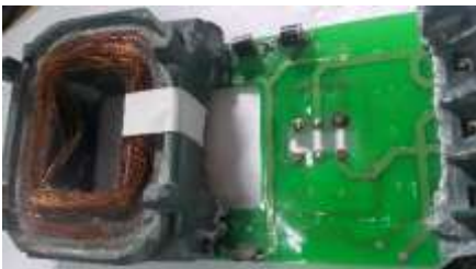
Fig.17.Inside contactor coil and it's equivalent circuit
