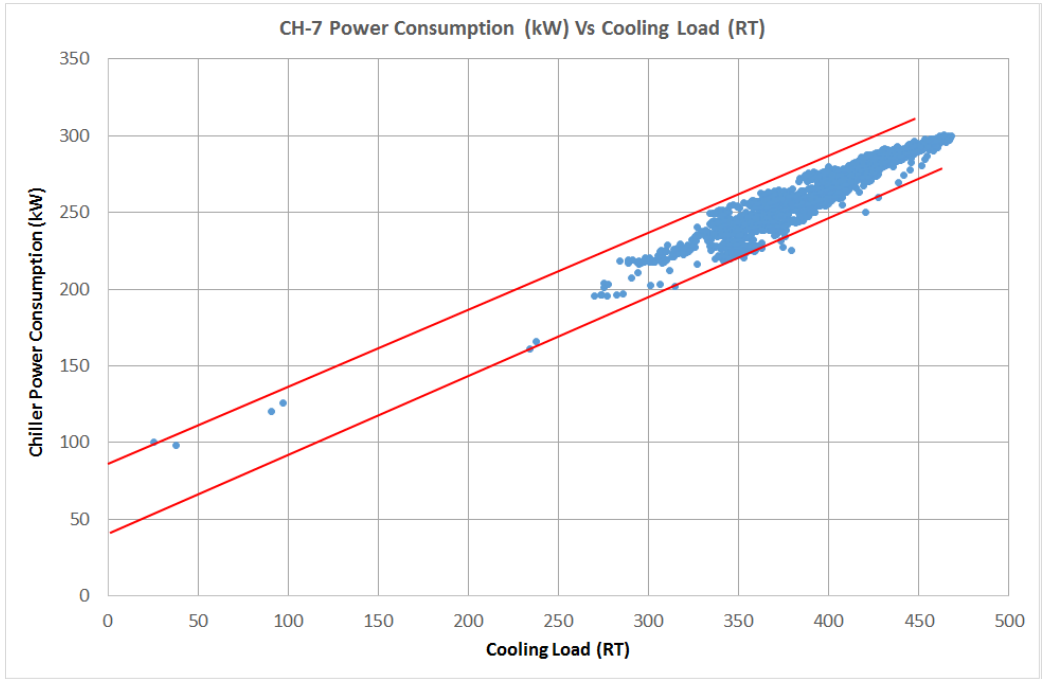
ပုံ - ၁၆ Power consumption Vs cooling load
