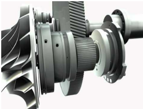
ပုံ ၄-၃၂ Centrifugal compressor integral gear and impellers
