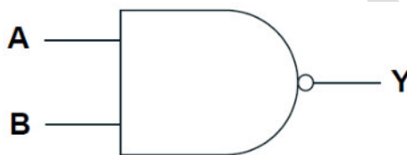
ပုံ 3-7. Two-input NAND gate and its truth table.
