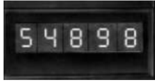
ပုံ 2-7(a) A seven-segment indicator field device (b) a thumbwheel switch.
