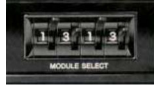
ပုံ 2-7(a) A seven-segment indicator field device (b) a thumbwheel switch.
