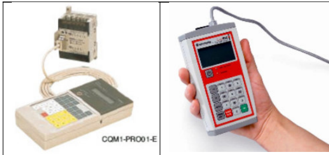
Figure 1-2. Small PLC with built-in I/O and detachable, handheld programming unit.
