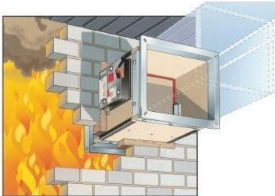
ပုံ ၅-၃၃ Fire rated partitions contain fire damage to the compartment of fire origin.
