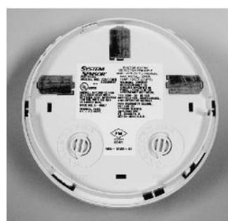
(ခ) Addressable smoke detector showing programming switches.
