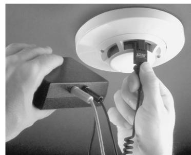
ပုံ ၈-၁၁ Manufacturer's calibrated test instruments
